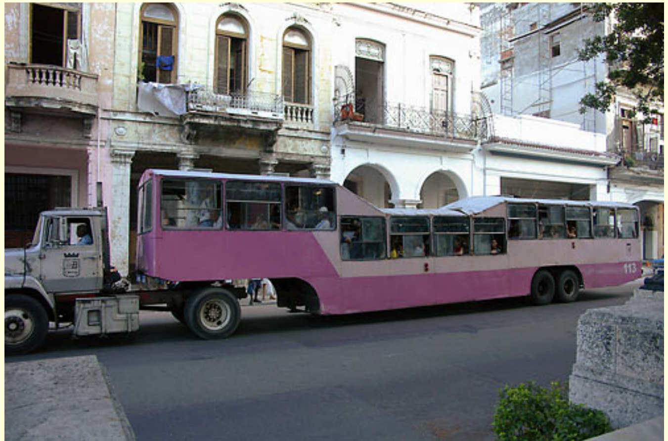
This unique Cuban transport vehicle, called a "camel", can carry 300 passengers. (Photo by John Morgan)
